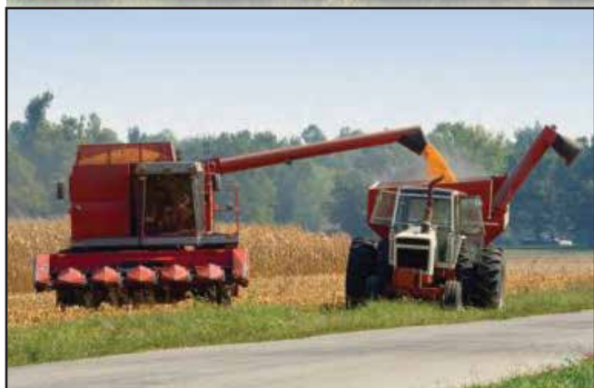
Look up! Equipment that can be extended, such as a grain elevator or stack mower, requires the utmost care when near a power line.
