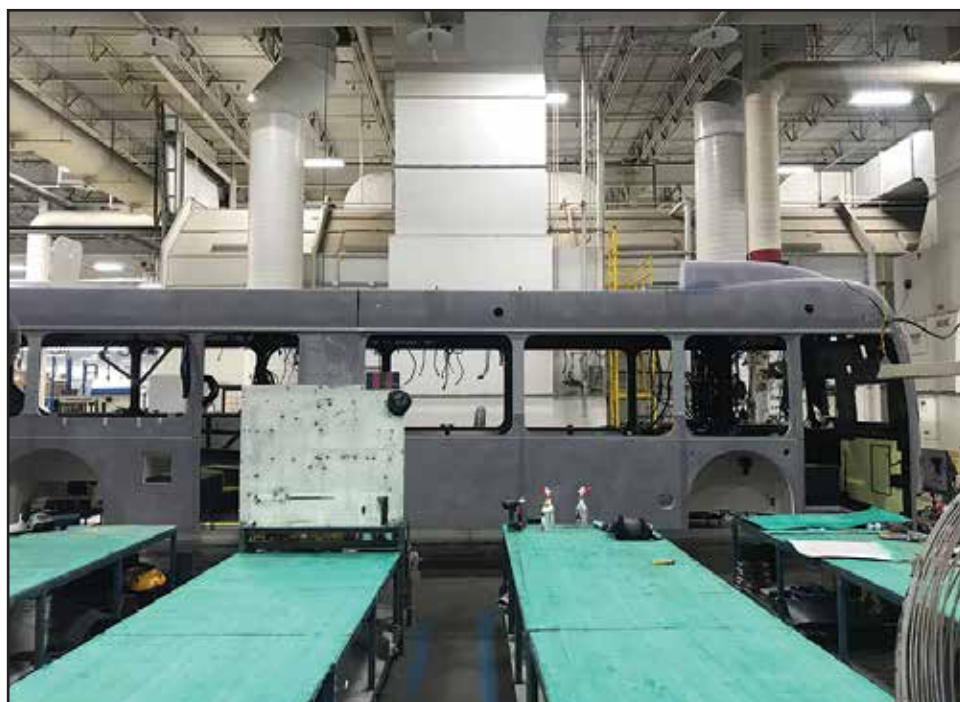
A new bus in the early stages of manufacturing. Wiring and internal mechanisms are being installed.
