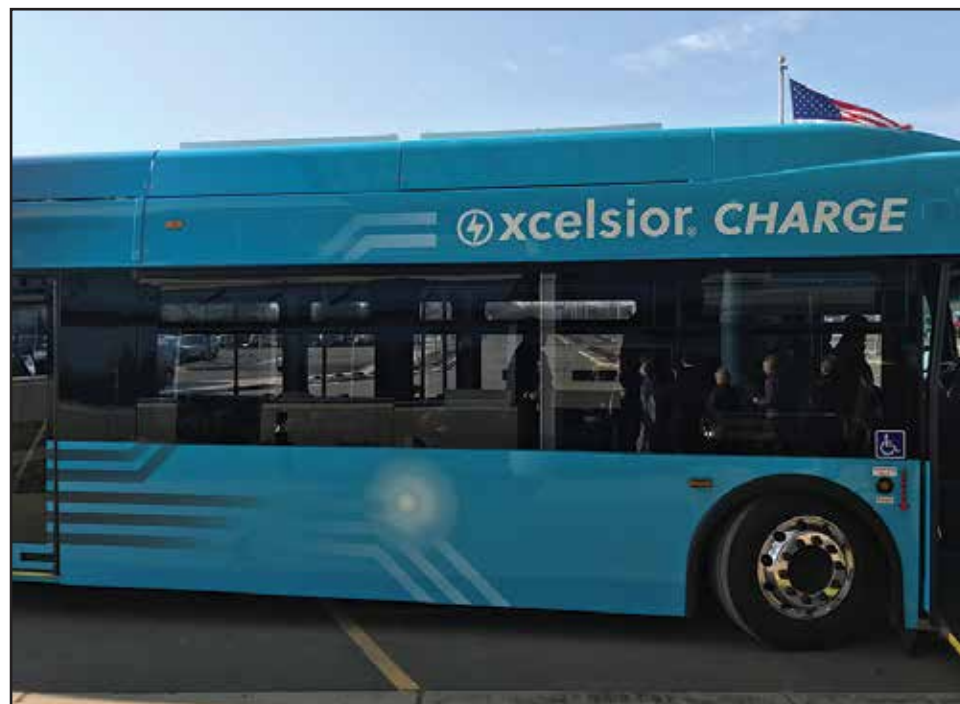
More than half of the C Line buses used by Metro Transit are fully electric, completely eliminating tailpipe emissions. The Xcelsior CHARGE — battery-electric buses were manufactured in St. Cloud, Minnesota by New Flyer of America.
