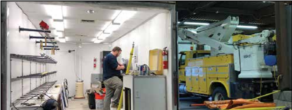
DG Energy Services- Dielectric Testing Division recently tested safety equipment used by line workers. The company brought their mobile trailer to the Co-op to test grounding equipment, hot sticks, insulated coverups and other protective equipment.
