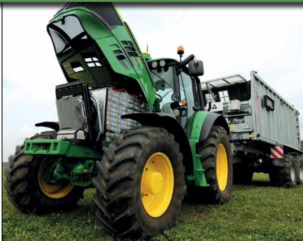
In 2017, John Deere showcased the first, fully battery-powered tractor. This technological innovation is truly the first of its kind. Nicknamed SESAM, for Sustainable Energy Supply for Agricultural Machinery, this all-electric tractor is modeled after John Deere's 6R series tractors.
