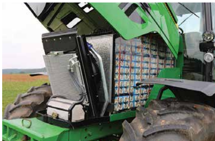
A peek under the hood of John Deere's first, fully battery-powered tractor. The all-electric tractor is modeled after John Deere's 6R series tractors.
