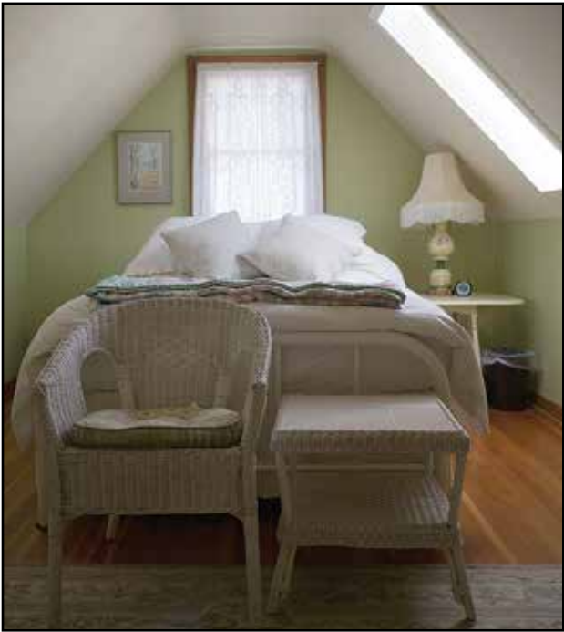
Converted attics tend to overheat in the summer because of low insulation levels and poor ventilation between the living space and the roof. A skylight can provide welcome daylight but unwanted solar heat gain. Photo Credit: Kevin Kerrick, Flickr.
