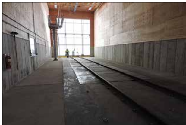
The train car pit can hold 60 ton of product at one time. All three train car hoppers unload at once and it takes only 5-6 minutes to unload an entire rail car.
