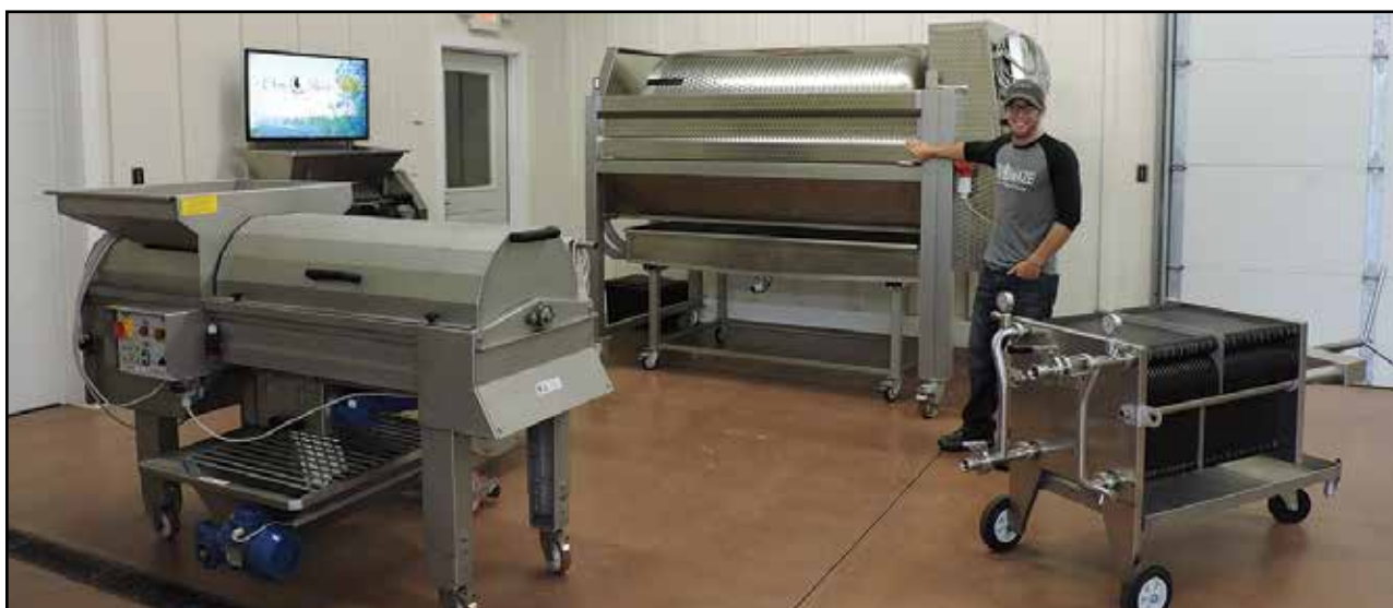
Long-time employee Lucas Gilhousen explained the machines used for crushing and removing grape stems and the larger wine press which can hold 2.5 tons of grapes.
