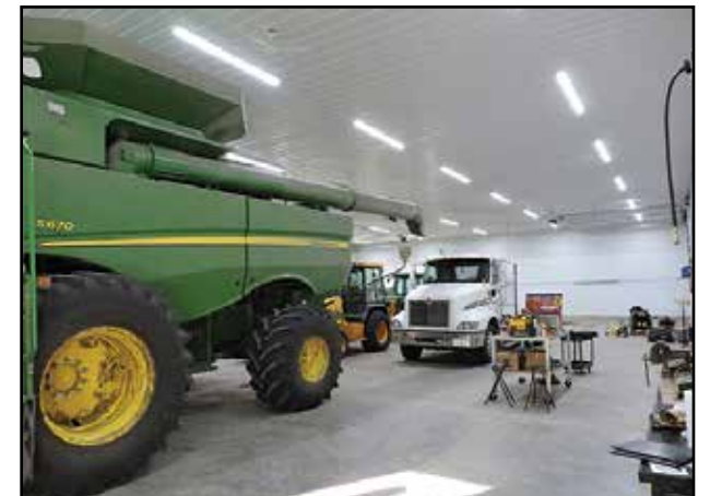
The interior of the shop utilizes eight-foot LED light fixtures that have six lamps each. The light fixtures are estimated to save about 42,000 kWh per year in electricity over standard lighting. Cost of the LED lights was just slightly more than standard fixtures after the rebate.
