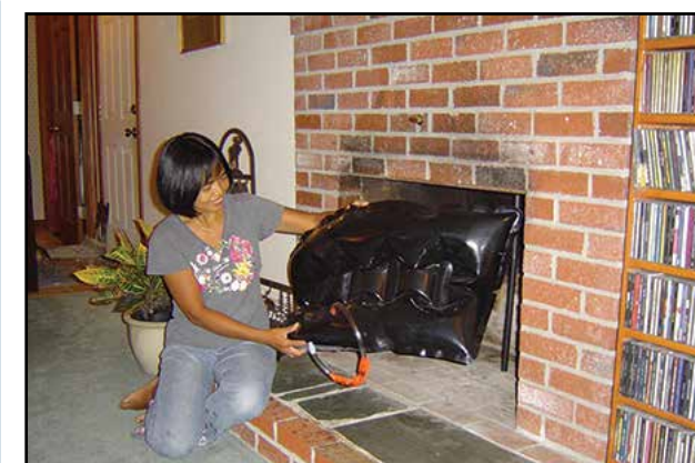
This Draftstopper chimney pillow is used to block indoor air leakage through the chimney when there is no fire. It is shown in its fully inflated state. In use, it is inflated after it is placed inside the flue.
