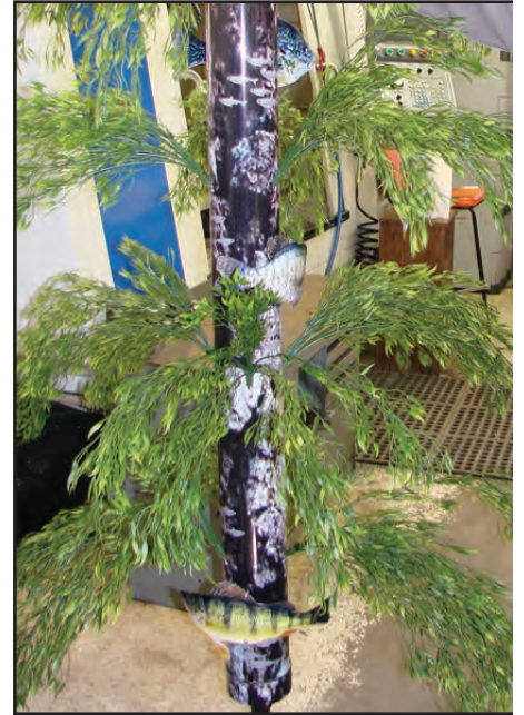
Deployment shaft. Fish decoys are mounted, then shaft is twisted to simulate swimming.
