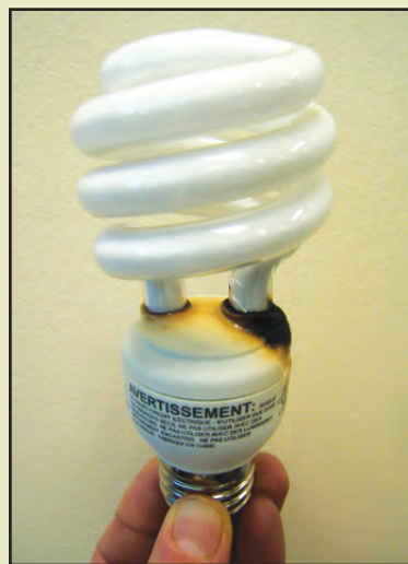
Sometimes the plastic at the base of a CFL will turn black as the bulb dims. This is normal in most cases because safety standards require use of special flame-retardant plastics in the base.
