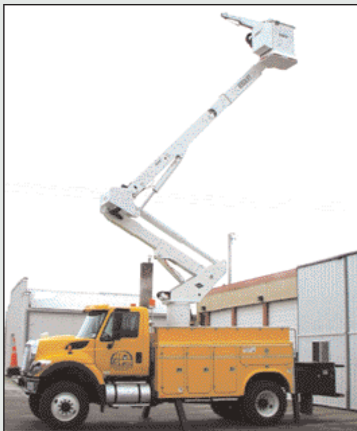
The newest truck added to the fleet has a working height of 54 feet. The boom can reach out 36 feet at 90 degrees.
