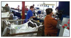
Employees of ATHC sort the different types of recyclables as they move on the conveyor line in front of them. Each person is responsible for pulling off a different type of product - plastic, glass, etc. Only the metal pop cans continue on through to a machine that crushes the metal.
